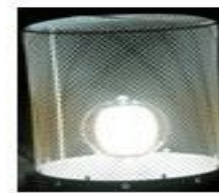
MW-induced plasma discharge
