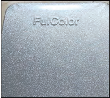
明显流痕 Obvious Flow lines Traditional Flake PE6001 60um
